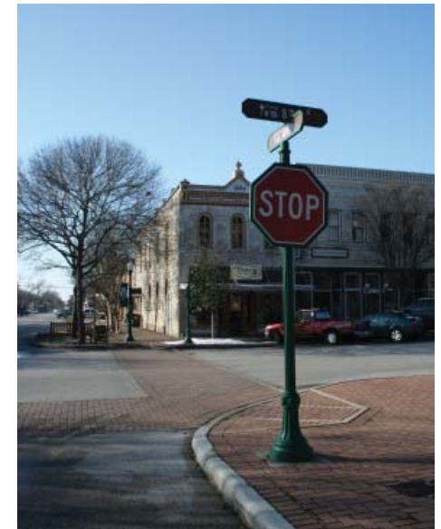
Pavers, curb cuts and stop signs create safer street crossings
